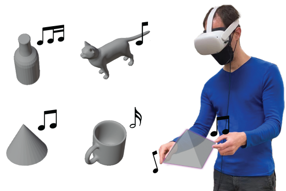
Figure 1: ShapeSonic allows users to touch virtual shapes in space by sonifying fingertip interactions. The VR headset is used solely for hand tracking and stereo audio. No visuals are shown to the user.
